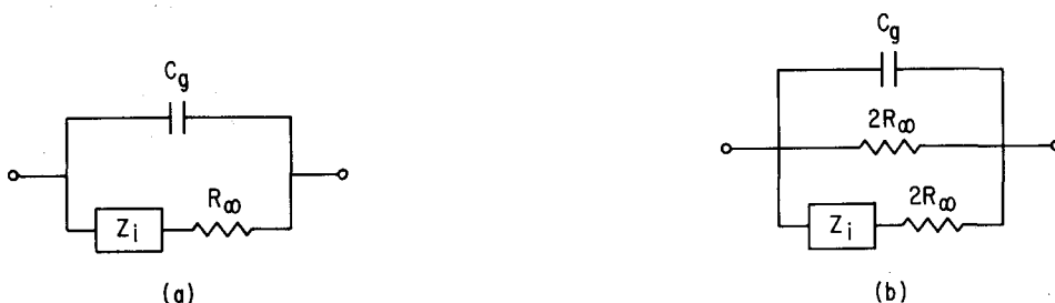
Fig. 1. Equivalent circuits for: (a) (0, 0) blocking case, (b) (0, \infty ) discharge case; no indifferent electrolyte present in either case.
