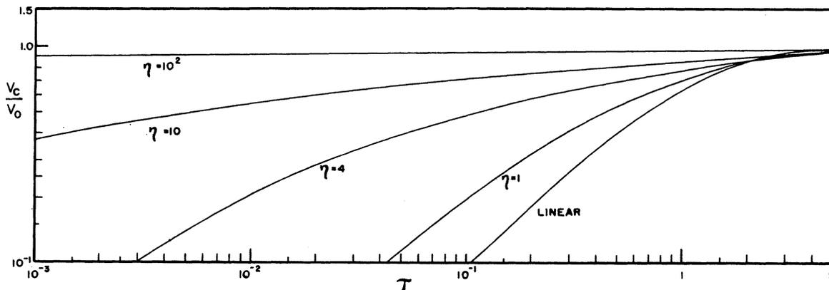
Fig. 2—Log-log plot of the charging of the exponential capacitor for various values of the applied voltage parameter  $\eta = \alpha V_0$ . The linear curve is for a normal voltage-independent capacitor.
