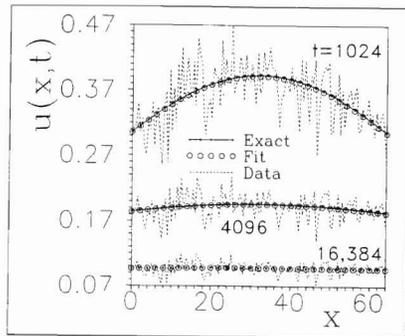
Figure 4. Data curves and points with  $\sigma_e=0.1$  proportional errors for  $t=1024, 4096, \text{ and } 16,384$ . For the noisy data, dotted lines connecting the discrete points have been included to guide the eye.
