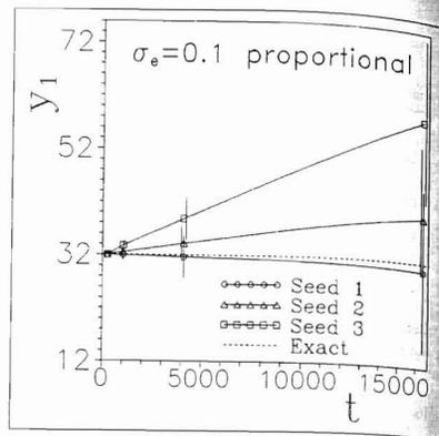
Figure 5. Dependence of inversion estimates of  $y_1$ , the line-source position estimate, on  $t$  for  $\sigma_e=0.1$  proportional-noise data for three different random-error seeds. The data for seed 1 are presented in Fig. 4. In order to allow the vertical lines showing the  $\pm$  one-standard-deviation range to be easily distinguished, those for seeds 2 and 3 have been displaced slightly to the left and right of their proper positions, respectively.
