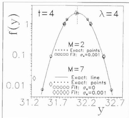
Figure 7. Comparison of the exact continuous source distribution and inversion estimates obtained with  $M=2$  and  $7$ , both with and without proportional errors present.
