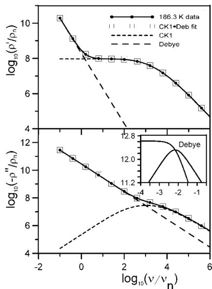
**Figure 2.** Log–log frequency–response plots of NMEC  $\rho'$  and  $\rho''$  186.3 K data and CK1•Deb-model fits. Also included are the separate CK1 and Debye responses calculated from the model fit parameters, as are low-frequency extrapolated results. The inset shows the calculated full Debye responses at lower frequencies. Here,  $\rho_n$  is 1  $\Omega$  cm.
