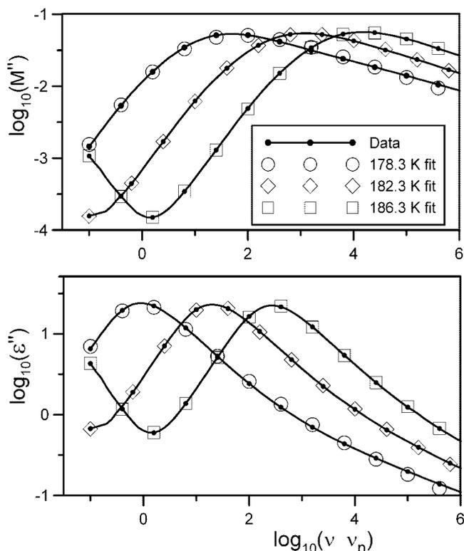
**Figure 1.** Frequency dependence of NMEC  $M''(\omega)$  and  $\varepsilon''(\omega)$  data and fits for various temperatures. To avoid overlap and add to clarity, only one out of every six data and fit points are shown, as discussed in section 3.1. The 186.3 and 182.3 K fits involved the composite model CK1•Deb results of rows 2 and 13 of Table 1, while the 178.3 K ones used the CK1• $C_S$  one. Here and elsewhere,  $\nu_n$  is 1 Hz.
