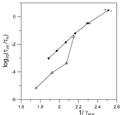
**Figure 5.** Plots of  $\log(\tau_{D0}/\tau_n)$  vs  $1/\gamma_{DCD}$  for NMEC (●) and glycerol (Δ) using the RCDCD·DC0 and CDCD·DC0 fit results in Tables 1 and 2. The lines are guides for the eye, and the normalization factor  $\tau_n$  is 1 s. The + symbols for the two most uncertain NMEC points were calculated using the standard deviation estimates of each of the relevant two fit parameters and define diagonal corners of the rectangular one-standard-deviation error box.
